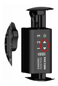
You can press , then quickly 2, or then quickly 2 to rotate MECHA-V by 90°.
