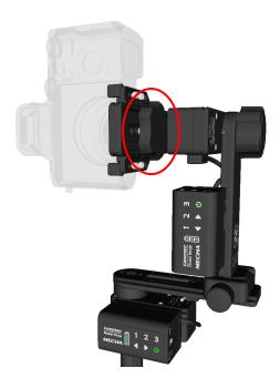
Plug the right shutter cable for the camera you are using into the Camera Port (CAM). This allows the shutter to be triggered automatically.
