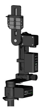
This code instructs the Combo to execute a panorama to the left or right, as follows: 12 shots around, 3 rows – at  $0^{\circ}$  and +/-  $45^{\circ}$  – plus zenith and nadir, starting from the **raised** position.
