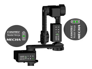
If a red LED is lit on the MECHA-V, this indicates that while the pairing is established, the firmware version is different from the one in the MECHA-H. Depending on the differences, some recently added features might not work.
