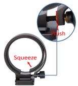
for trouble shooting. Squeeze to take out the inner ring. Check label on inner ring to confirm with lens in use and direction of mounting. The arrow should point to the front of lens.
