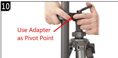
Tighten the knob at the side of upper adapter. This will align the upper and lower adapters. Hold the upper adapter and slowly tighten the top mounting knob to prevent twisting. Use the upper adapter as pivot to fully tighten the knob.
