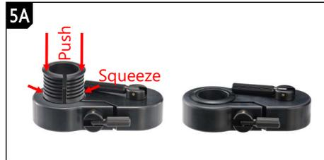
To use Pole 1 or Pole 2 upper unit on tripod adapter, the fitting must be installed. Loosen the side knob. With the flange facing up, squeeze and push the fitting into the adapter. The fitting should snap in place. Then continue to **Step 6**.
