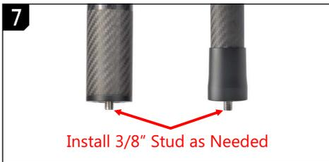
Install a 3/8" x 3/4" stud (from the pole package) at the base of pole using the included hex key, except when a Pole Rotator is mounted on the lower adapter, or when a motorized rotator is to be used atop a pole. Tighten the stud fully to prevent loosening.
