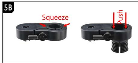
To use Pole 2 lower unit on tripod adapter, the fitting (if any) must be removed. Loosen the side knob. With the flange facing down, squeeze and push the fitting out of the adapter. Then continue to **Step 6**.
