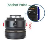
Align window on the inner ring to the reference mark of the focus scale. Insert the lens. Stretch the ring when necessary. Move it to a position where it fits snugly. Push it against the anchor point on lens to ensure exact mounting and consistent NPP setting.
