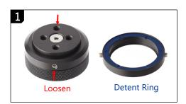
Loosen two set screws on the detent ring till it can be removed from the rotator. On new detent ring, apply a thin layer of grease to the area indicated. Loosen set screws so that it can be mounted on the rotator. Clean the grease on the old detent ring and store it safely for future use.
