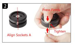
Turn the top part of the rotator to roughly align sockets **A** to the detent click ball. Mount the new detent ring. Align the set screws to the click ball. Press the ring firmly near the click ball. Tighten the set screw. Press the ring firmly near the other set screw. Tighten the set screw to finish the operations.
