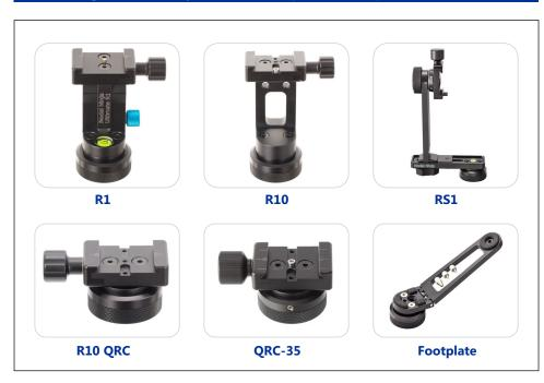
Install Nodal Ninja Ultimate R1/10, R10 QR clamp, QRC-35, Nodal Ninja RS1, or Rotator Footplate on Rotator Mini by means of two M5 flat head screws, which are supplied in the corresponding package. For best appearance, choose an orientation so that the text markings is at a less visible position.
