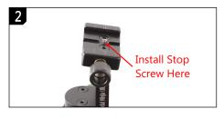
Install the stop screw (came with the stop plate) at the middle socket on the QR clamp. Remove any other safety screw installed. Mount the lens ring on the clamp. Slide until it falls into the stop. Confirm the NNP reading is 1.8 (or 1.825 more precisely).
