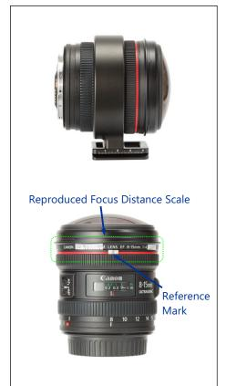
Manual focus is preferred for making stitched panos. Turn the **AF/MF** switch to **MF**. The focus distance scale will be hidden by the lens ring. Users can use live view to set a focus distance where the distant and near objects are both in focus.
