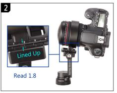
Slide the lens ring plate (LRP) to the NPP setting. There are 3 lines marked on the QR clamp. Use the center line for distance reading. Other lines are 1.5mm apart from the center line. Use them to assist reading to an accuracy of 0.5 mm. Use the side opposite to the QR handle for best accuracy.
