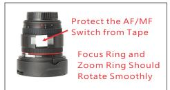
Fix the inner ring with a piece of tape about 40mm (1.5") long. Stretch the tape so that the ring will grasp the lens firmly. Cut any tape that goes beyond the chamfered area on either side of the slit. Test that focus ring and zoom ring rotate smoothly. If not, nudge the inner ring slightly away from the hindered focus ring or zoom ring and test again.
