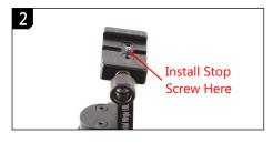
Install the stop screw (came with the stop plate) at the middle socket on the QR clamp. Remove any other safety screw installed. Mount the lens ring on the clamp. Slide until it falls into the stop. Confirm the NNP reading is 1.4.
