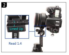
Slide the lens ring plate (LRP) to the NPP setting. There are 3 lines marked on the QR clamp. Use the center line for distance reading. Other lines are 1.5mm apart from the center line. Use them to assist reading to an accuracy of 0.5 mm. Use the side opposite to the QR handle for best accuracy.
