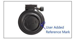
Align the outer ring to the slit of inner ring. Insert the outer ring (loosen its knob further if needed) from the back of the lens. Tighten its knob slightly. Rotate the outer ring so that it snaps to the inner ring and rotates smoothly. Optionally align the notch indicated to the user added reference mark. Tighten the knob fully.
