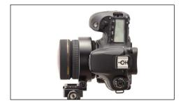
Mount the lens to the camera and it is now ready for use on any Arca Swiss compatible gear. The camera will be in portrait mode with handgrip pointing up. Loosen the knob on the ring to rotate to other angle. Use the notches (at 30° interval) at the back of ring to have accurate roll angle alignment. Use the center of **AF/MF** switch as the reference.
