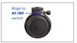
Align the outer ring to the slit of inner ring. Insert the outer ring (loosen its knob further if needed) from the back of the lens. Tighten its knob slightly. Rotate the outer ring so that it snaps to the inner ring and rotates smoothly. Align the notch below the lens ring plate to the **AF/MF** switch. Tighten the knob fully.
