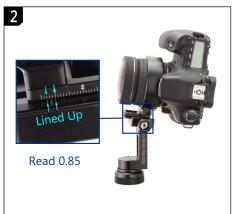
Slide the lens ring plate (LRP) to the NPP setting. There are 3 lines marked on the QR clamp. Use the center line for distance reading. Other lines are 1.5mm apart from the center line. Use them to assist reading to an accuracy of 0.5 mm. Use the side opposite to the QR handle for best accuracy. NPP setting of Sigma 8mm F3.5 for Canon is 0.85. Check that the LRP has "LRP40" labeled at the base.
