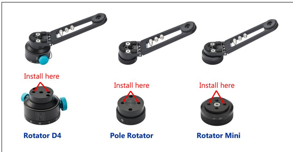
Pole Rotators, Rotator D4 and the Rotator Mini have two M5 sockets separated by 22mm. Foot plate can be attached to them by means of two M5 flat head screws.
