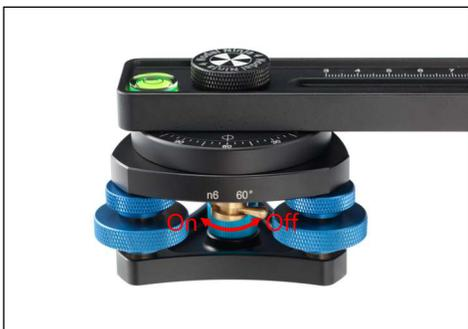
Turn on/off a detent option by flipping the switch to the left/right respectively. To use a detent option, turn on its switch and turn off the others. More detent options are available by skipping one or two click stops. When transporting the tripod with Nodal Ninja RD3L mounted, rotate the RD3L to 0 degrees and turn on all the detent switches to enable stronger resistance to rotation.
