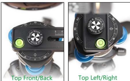
Confirm the accuracy of reading by ensuring the bubble is centered horizontally when viewed from the top front/back as well as from the top left/right. If not, re-adjust roller(s) to center the bubble. Lock the level locks to prevent accidental change of level. Do NOT change the level for remaining shots in the same pano sequence.
