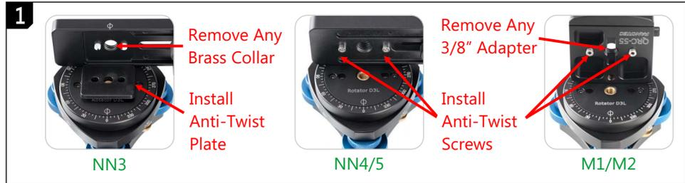
For NN3, remove brass collar (if any) installed on the lower rail. Align and place the anti-twist plate on RD3L.
