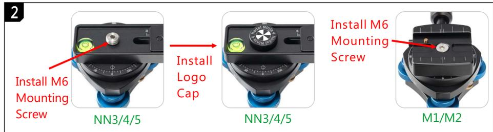
Align the anti-twist plate/ sockets and place the lower rail or QRC-55/65 on RD3L. Install and tighten the M6 mounting screw using a 4mm hex key. For NN3/4/5, install the logo cap on the mounting screw. Now the Nodal Ninja with RD3L is ready for use.
