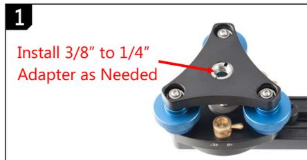
Install the 3/8" to 1/4" adapter if the tripod has a 1/4" thread. If tripod top plate has bare metal surface, consider adding a friction material to prevent loosening and/or scratching the base of RD3L. An optional cork sheet is available from Fanotec.
