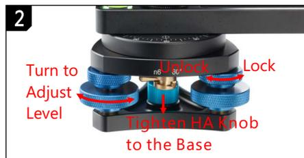
Place the tripod legs in their preferred positions. Unlock the level locks. Turn the rollers to roughly the middle of their full adjustment range. Tighten the "Head Alignment Knob" (HA Knob) of RD3L to the base. Tighten RD3L to tripod while holding the knob with fingers.
