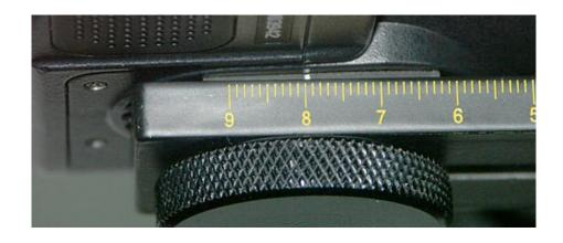
Check that the lens axis is parallel to the vertical rotator arm then tighten the knob. Check if the whole assembly is leveled. Then you can start taking photos at various angles of elevation and rotation.
