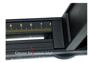
So, for a Dimage 7, you slide the vertical arm to 60.5mm because you must use the offaxial adapter for it. For an E20, you slide it to 51mm if you use the off-axial adapter or to 45mm if you use the EPDM adapter plate.
