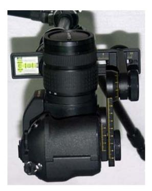
Slide the camera to the correct position, taking the off-set by the adapter into account. Again take the choice of the adapter into account for the horizontal adjustment. Level the assembly and start shooting.
