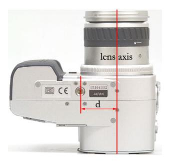
Using the Dimage 7 as an example, first, you need to determine the lens axis. This can sometimes be difficult. But most of time, there are reference point that lies on the lens axis. For example, the 2 screws under the lens of Dimage 7 lie exactly on the lens axis. Try to find some similar reference points on other cameras. If there is none, draw a line (with pencil) that bisects the lens as accurately as possible. Then measure the distance from the center of tripod socket to
