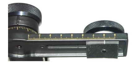
On the adapter, there are white marks that correspond to the center of tripod mount. So you simply mount your camera on it and adjust its position so that the white mark corresponds to the distance of the tripod mount from the entrance pupil position.
