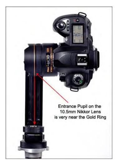
Insert a rail stop as shown and tighten to lock, and remember this position. The upper position is now set, unless you change camera and / or lenses or vary the focal length, it will remain as is.
