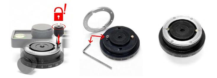
Using the enclosed hex key loosen the inner hex screw enough to release detent ring. Some units may have the hex key tool located inside the tension knob, as shown above left. Place the detent ring with desired side face up. Tighten hex screw and reassemble.
