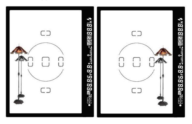
Now rotate the camera so the two objects are now in the right side of the viewfinder frame. Go back and forth a few times, and watch to see if the distance between the two poles changes. If the distance changes, even slightly, then you have parallax and you'll need to move the camera and lens slightly forward (or back) on the upper rail.
