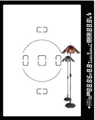
Now rotate the camera so the two objects are now in the right side of the viewfinder frame. Go back and forth a few times, and watch to see if the distance between the two poles changes. If the distance changes, even slightly, then you have parallax and you'll need to move the camera and lens slightly forward (or back) on the upper rail.
