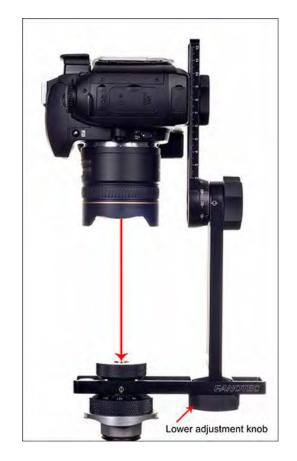
Insert a rail stop as shown and tighten to lock, and remember this position. The lower position is now set and will not change regardless of lens or focal length.
