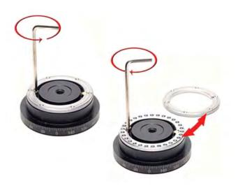
Using the enclosed hex key loosen the inner hex screw enough to release detent ring. Some units may have the hex key tool located inside the tension knob, as shown above left. Place the detent ring with desired side face up. Tighten hex screw and reassemble.
