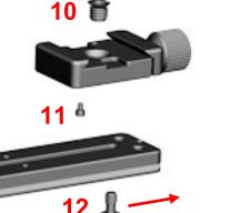
Slide the 1/4" screw and hence QRC-40A far most 13. Slide QRC-35 to far left or right so that it is flush with plate 13 below. Tighten the knob on QRC-35.
