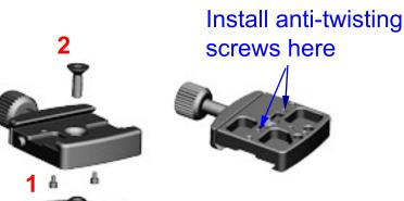
3. Attach MFR-Dovetail 35 to the end of MFR-160, by using 2 M5 screw with brass fitting.
