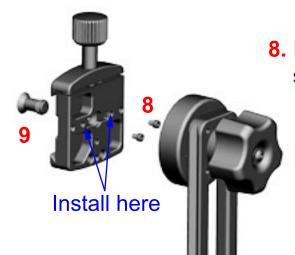
8. Install 2 anti-twisting screws on the QRC-55.
