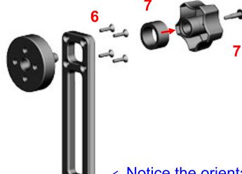
Press the plastic fitting to the upper rotator tightening knob. Tighten the knob to the upper rotator and then install the knob retention screw.
