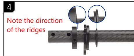
4 Insert the bearing cover, housing (with fitting in case of Pole 2) and base mount into the pole section. Note the direction of parts. The side with protruded ridge should be facing the bearing housing.
