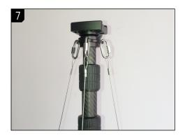
Any support wire/rope can be attached to holes on the bearing housing to as guy wires or safety wire. For best result, use inelastic wires.
