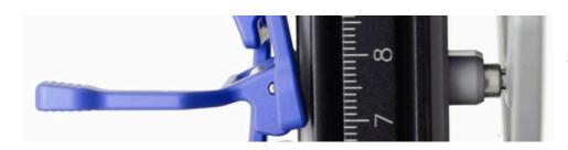
Stopping plunger in action. Front pin engaged.
