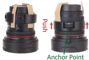
Stick the brown backings back to the tapes with slippery side facing the tape and die cut area away. Bend to crimp the backing, uncovering half of the tape.
