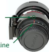
There is no feature on lens to aid setting accurate roll angle of camera apart from 0° (landscape) and 90° (portrait). A piece of label can be added near the Limit switch as a reference mark. Alternatively, rotate the zoom ring to align a nearest ridge on the rubber ring to the reference line. Align the 90° notch to the reference line with the help of rubber ridge. Tighten the knob securely. Mount lens to camera.
