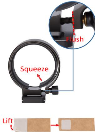
Loosen the knob on outer ring until the edge of opening is flush with lens ring plate. Don't loosen further. It will only make installation more difficult and can potentially damage the thread if knob is completely unscrewed. See Page 2 for trouble shooting.
