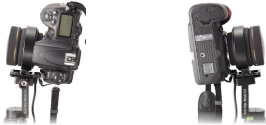
It is reported that lens ring for Sigma 8mm for Nikon blocks the remote port for Nikon D200/300/700 etc.
