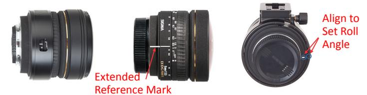
There is no feature on lens to aid setting accurate roll angle of camera apart from 0° (landscape) and 90° (portrait). A piece of tape or label can be added to extend the reference mark on the lens. Roll angle can then be read in 30° intervals by aligning this mark to notches at the back of outer ring.
