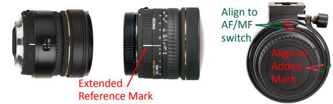
Roll angle of camera can be set relative to the AF/MF switch on lens. More accurate value can be obtained by extending the reference mark on the lens using a piece of tape or label. It can be read in 30° intervals by aligning notches at the back of outer ring to AF/MF switch or the added mark.
