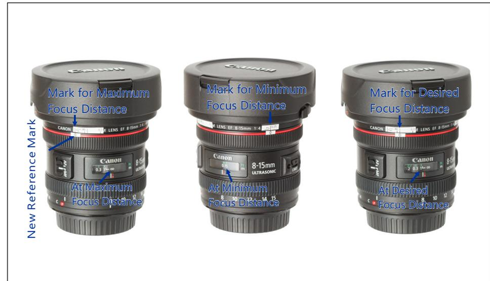
The lens uses USM motor for auto focus. The focus ring is not rigidly linked to the focus mechanism. That means the ring can still be rotated after reaching the limits of the focus distances. This presents a challenge in reproducing the scale. One workaround is to reproduce the whole range including the maximum and the minimum and turn the focus ring in a special manner described below.
