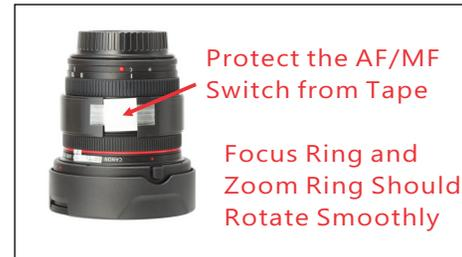
Fix the inner ring with a piece of tape about 40mm (1.5") long. Stretch the tape so that the ring will grasp the lens firmly. Cut any tape that goes beyond the chamfered area on either side of the slit. Test that focus ring and zoom ring rotate smoothly. If not, nudge the inner ring slightly away from the hindered focus ring or zoom ring and test again.
