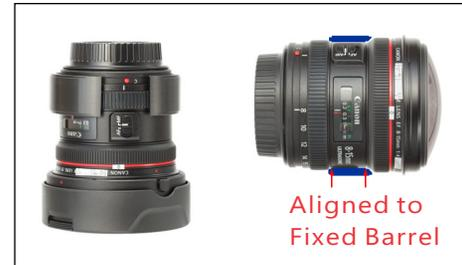
Align the slit of the inner ring to **AF/MF** switch on lens. Stretch the ring to pass over the zoom limit switch. Position it evenly between the focus ring and zoom ring. Use the cross section of slit for alignment. Keep even spacing between the slit and **AF/MF** switch. Place a piece of paper to cover the AF/MF switch to protect it from glue of tape.
