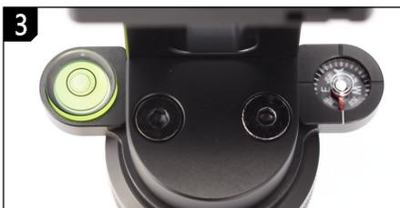
To orient the panorama in the map, move the tripod so that the red pointer aligns with the white mark on the compass. Now the camera is pointing to the North. Look at the compass from the front for best reading accuracy.
