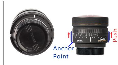
Align the slit on the inner ring to the left of the focus scale. Insert the lens. Stretch the ring when necessary. Move it to a position where it fits snugly. Push it against the anchor point to ensure reproducible mounting and consistent NPP settings.
