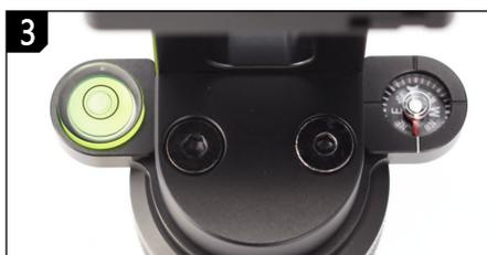
3 To orient the panorama in the map, move the tripod so that the red pointer aligns with the white mark on the compass. Now the camera is pointing to the North. Look at the compass from the front for best reading accuracy. Level the R10 head by adjusting tripod legs or a level adjustment device.
