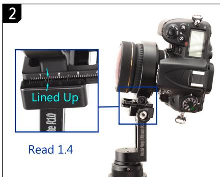
2 Slide the lens ring plate (LRP) to the NPP setting. There are 3 lines marked on the QR clamp. Use the center line for distance reading. Other lines are 1.5mm apart from the center line. Use them to assist reading to an accuracy of 0.5 mm. Use the side opposite to the QR handle for best accuracy. NPP setting for 4 shots around is 1.4. Check that the LRP has "LRP45X" labeled at the base.
