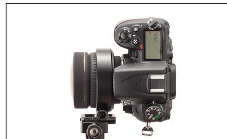
Mount the lens to the camera. Loosen the knob on the ring to align the LRP to the lens release button on the camera. The camera will be in portrait mode with handgrip pointing up. Loosen the knob on the ring to rotate to other angles. Use the notches (at 30° interval) at the back of ring and the added reference mark for accurate roll angle alignment.
