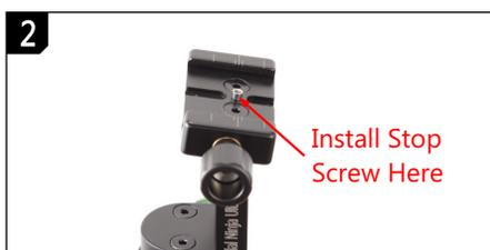
2 Install the stop screw (came with the stop plate) at the middle socket on the QR clamp. Remove any other safety screw installed. Mount the lens ring on the clamp. Slide until it falls into the stop. Confirm the NNP reading is 1.4.
