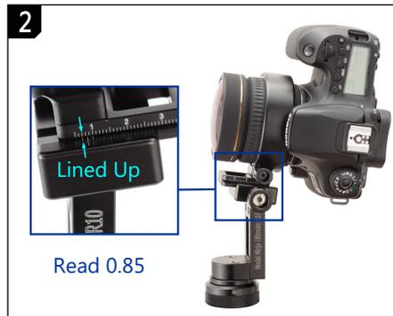
Slide the lens ring plate (LRP) to the NPP setting. There are 3 lines marked on the QR clamp. Use the center line for distance reading. Other lines are 1.5mm apart from the center line. Use them to assist reading to an accuracy of 0.5 mm. Use the side opposite to the QR handle for best accuracy. NPP setting for 4 shots around 0.85. Check that the LRP has "LRP40" labeled at the base.
