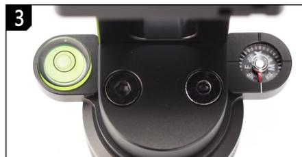
To orient the panorama in the map, move the tripod so that the red pointer aligns with the white mark on the compass. Now the camera is pointing to the North. Look at the compass from the front for best reading accuracy. Level the R10 head by adjusting tripod legs or a level adjustment device.
