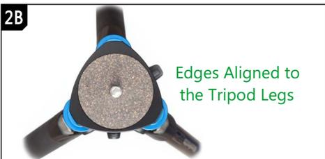
Alternatively, HA Knob allows EZ-L II to align its edges to the tripod legs to minimize the nadir footprint. Loosen EZ-L II a bit. Gradually loosen HA Knob while tightening EZ-L II, until its edges are about to align with the tripod legs. Then tighten EZ-L II fully.
