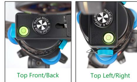
Level the bubble as described in previous section. Confirm the accuracy of reading by ensuring the bubble is centered horizontally when viewed from the top front/back as well as from the top left/right. If not, re-adjust roller(s) to center the bubble. Now the bubble is leveled.
