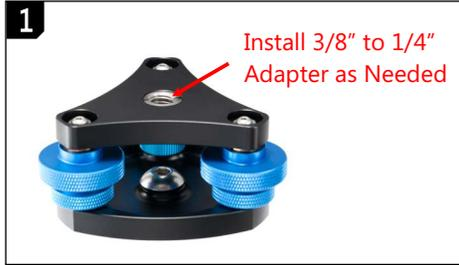
Install the 3/8" to 1/4" adapter if the tripod has a 1/4" thread. If tripod top plate has bare metal surface, consider adding a friction material to prevent loosening and/or scratching the base of EZ-L II. An optional cork sheet like that on EZ-L II is available from Fanotec.
