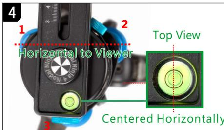
Stand in a position so that 2 rollers (1 and 2) are horizontal in front of you. Look at the bubble from vertically above. Adjust the horizontal rollers to center the bubble horizontally.
