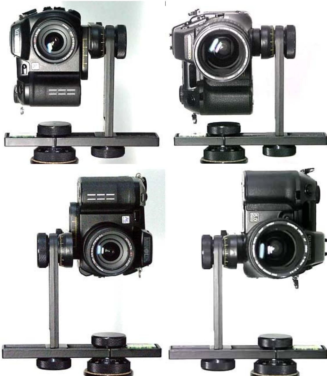
It has all the import features to allow you to rotate your camera about the entrance pupil position (commonly mistaken as the nodal point) of the lens. These include horizontal adjustment, axial adjustment (along the lens axis) and adjustment for off-axial tripod mount.
