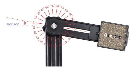
The upper rotator can be installed with an offset of +/- 5, 7.5, or 10 degree from the horizon, making it perfect for single row spherical panoramas with various fisheye lenses.
