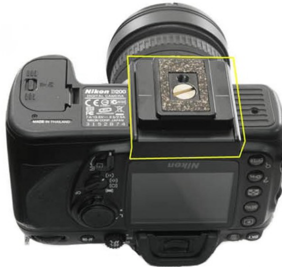
Attach camera plate to camera.
