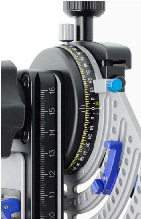
Rotate the index ring by 180 degrees. Align the 0 degree mark accurately and tighten the light blue screws to fix the index ring.
