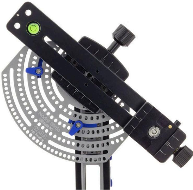
Point the camera to the upmost region of interest without touching the lower rotator. Engage the stopping plunger by lifting the lever. Loosening the end tab handle and slide the stopping tab against the vertical rail stop and tighten. This sets the upper limit and ensures camera and lens will not inadvertently touch the pano head during up and down rotation.
