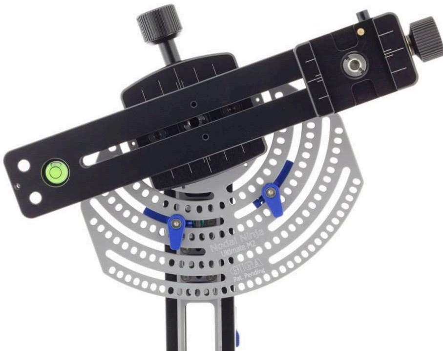
Point the camera to the lowest region of interest without touching the lower rotator. Engage the stopping plunger by lifting the lever. Loosening the end tab handle and slide the stopping tab against the vertical rail stop and tighten. This sets the lower limit and ensures camera and lens will not inadvertently touch the pano head during up and down rotation.
