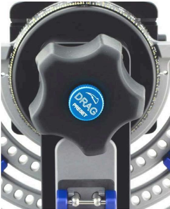
The upper rotator tightening knob adjusts the friction for rotation of upper rotator and locks the rotator when fully tightened. A proper level of friction provides smooth movement at the upper rotator when using as a gimbal head, useful when tracking moving objects such as in sporting events or wildlife. It also helps to align the rotator to the indexing stops more precisely.
